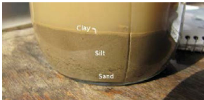
Figure 3. Jar with water used to separate soil into clay, silt, and sand to determine percentages.
